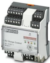
EV charge control is used to charge electrical vehicles on the 3-phase AC mains power supply according to IEC 61851-1 Mode 3. All necessary control functions are integrated. Additional functions are available for various charging applications.
