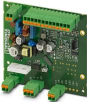
The EV-CC-AC1-M3-CC-SER-PCB-MSTB charging controller as a PCB for charging electric vehicles according to IEC 61851-1, Mode 3, optimized for charging stations with permanently mounted Vehicle Connector. Connection via PCB connector on header.
